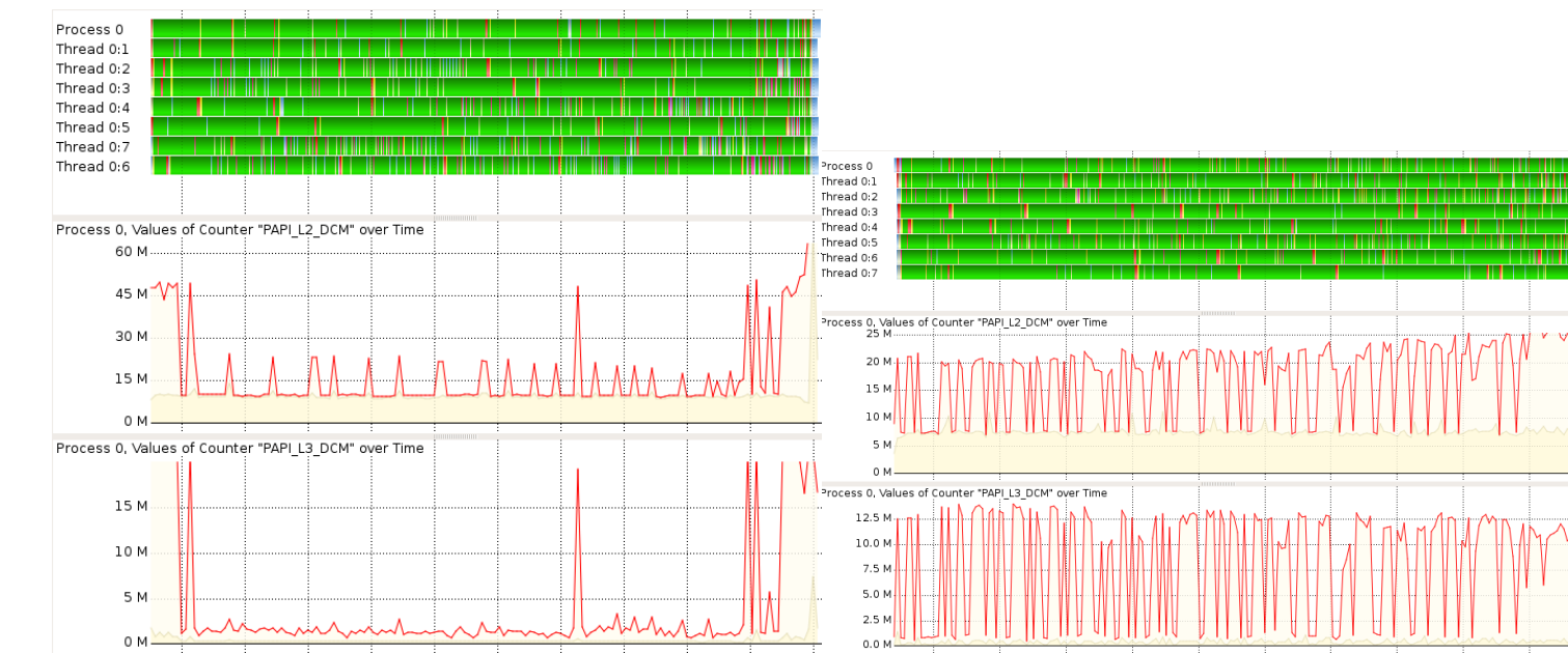
Figure 2: Timelines along with L2 and L3 cache misses. (a) Scheduling with Locality Tags: Reasonable cache locality, but limited load balance. (b) Scheduling with Locality Tags and Work-stealing: Reasonable load balance, but low cache locality.
